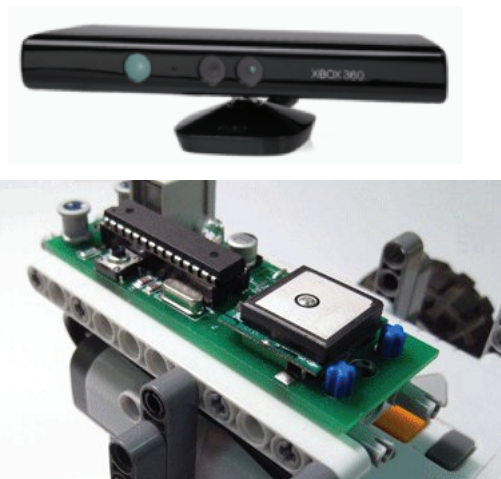
Fig. 1.6 Some additional sensors that we could use such as the Microsoft Kinect and a GPS for the Lego NXT.
