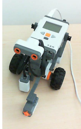
B. Tribot with ultrasonic, touch and light sensor
