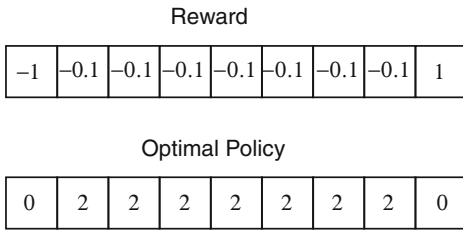
Fig. 18 Example of using policy iteration on a chain of rewarded states. Left reward values and optimal policy for each state, where a policy value 1 means “go left” (not present) and a value 2 means “go right”. No further action is taken in the end states
