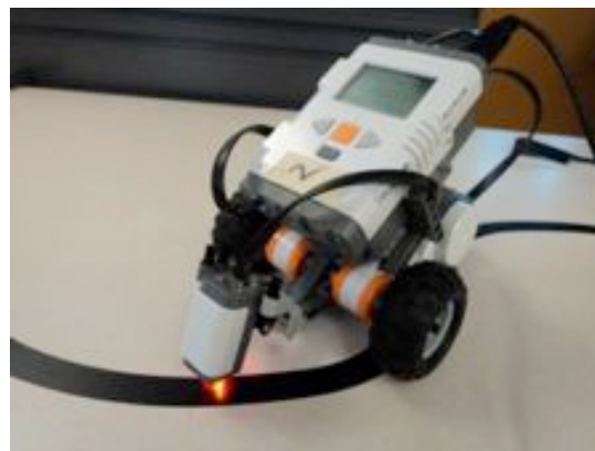
Fig. 2.4 Basic Lego Robot with microprocessor, two motors, and a light sensor.
