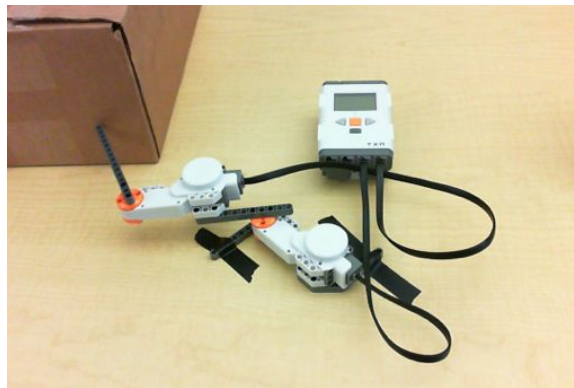
Fig. 2.8 (A) A simple robot arm with two joints that can point at an obstacle.
